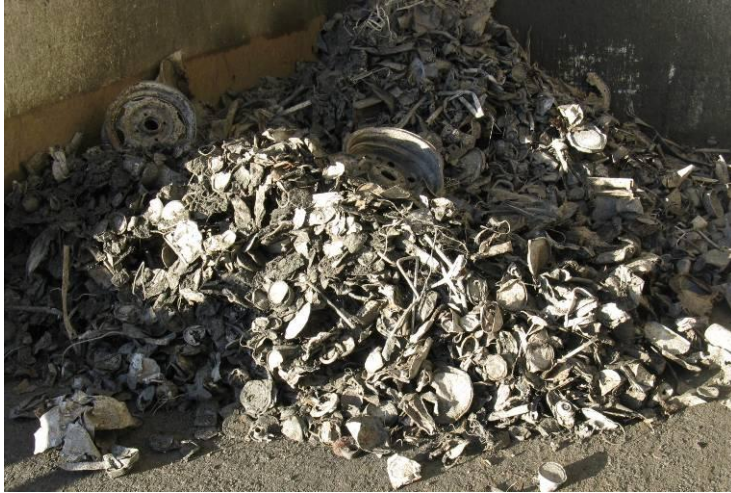
Figure 4-9: Ferrous Metals Separated from the Slag of a MSW Incinerator by Means of a Magnet
