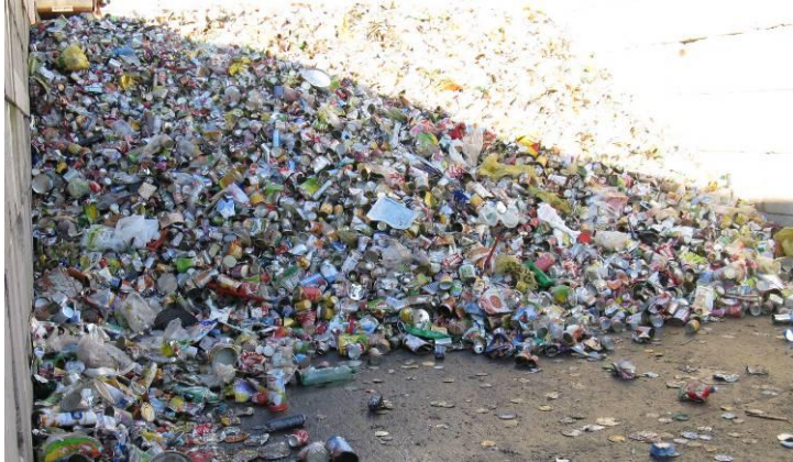
Figure 4-7: Ferrous Metal Cans Separated from “Yellow Bag” Collection (same Collection Material as shown in Figure 4-6) by means of a magnet
